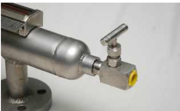
Vent valve for 300# application magnetic level gauge in forged SS316L construction
